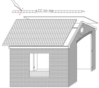
Fit the prepared roof panels to the goods shed. Cover the ridge with LCC 00-09 roof ridge tiles which need to be cut to length.
