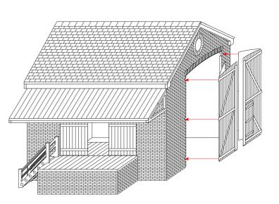
Fold the train gates LCC 04-02 and LCC 04-03 in half with some watered down glue between. Make sure to align them neatly and press them for a few minutes between something heavy so they bond well and are flat.
