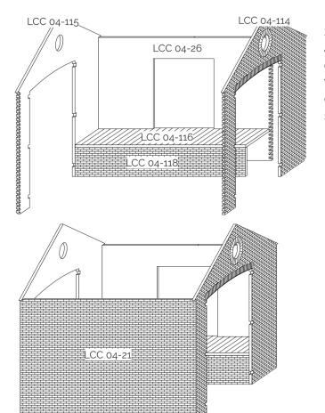
Start by joining LCC 04-26 with LCC 04-114 and LCC 04-115. Make sure to glue in the gate panels as shown on the diagram. The wider parts should be facing the loading door. Fit the inner platform which will stabilise the construction.
