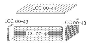
Assemble the loading platform.
