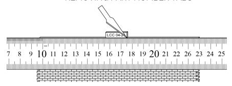
Using a ruler (ideally flat steel one) remove tabs from the parts. Use multiple light passes with a sharp hobby knife. Tab placement is usually in an area that will be covered with something so small imperfections in cuts are usually not a problem.
