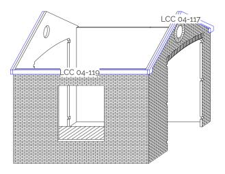
Glue the barge boards LCC 04-117 to the gate panels making sure they are well aligned with the slopes of the gable.
