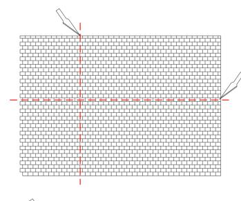
Trim the roof panels LCC 00-24A and LCC 00-24B to size. They should end up approximately 94mm wide and 51mm high. Make sure to cut them oversized at first and then fit to exact size. Roof panels should be resting with the edge touching the facia boards and the ends should be flush with the barge boards.
